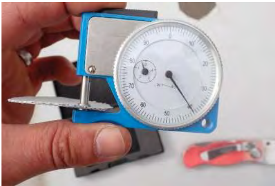
Photo No. 26 - The existing JP Stevens single-ply Hypalon roof membrane was noted to be a 40-mil (0.04-inch) thick single-ply, reinforced with a polyester-fabric scrim.
