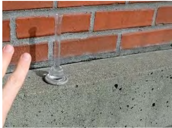
Photo No. 92 - Depicts testing conducted at the horizontal surface of the concrete foundation wall at the South Elevation of the building. This area was chosen due to the proximity of relatively moist-appearing mortar at the interface with the concrete. The small amount of moisture absorption exhibited at this location (0.2 after 30 minutes) indicates relatively high moisture penetration resistance, even in an area where water might be expected to pool and degrade the concrete in an accelerated manor.
