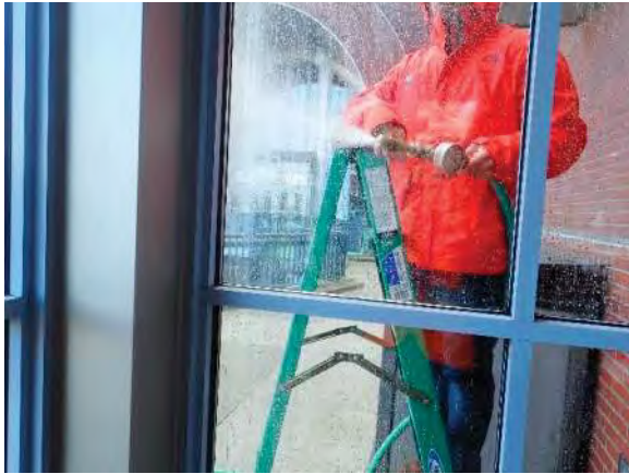
Photo No. 109 - Depicts the storefront window system during testing, as viewed from the interior. No water was observed penetrating to the interior during the test of this windows', sill, jambs, and the head, as well as its sealant joints. Thermographic imaging did not indicate any moisture penetration during the testing (see next image).
