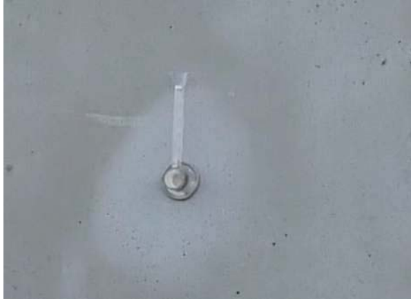
Photo No. 93 - Depicts RILEM testing at the face of the concrete foundation wall at the East Elevation of the building. The area around the tube was bristle-brush cleaned prior to testing to ensure proper adhesion by the RILEM Tube. The concrete foundation wall locations tested generally exhibited high levels of moisture penetration resistance.
