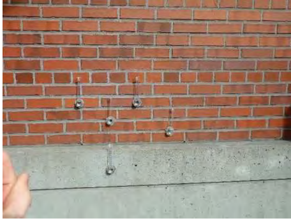
Photo No. 89 - Depicts overview of RILEM testing at the South Elevation adjacent the parking lot. This area exhibited strong resistance to moisture penetration at all the tested masonry and concrete surfaces.
