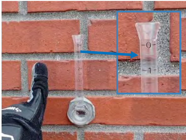
Photo No. 91 - Depicts close-up of the specimen on the West Elevation that exhibited among the most moisture penetration at 0.5 after the 30-minute test. While this does indicate good water-penetration resistance, the increased absorption will lead to an increased rate of water-related degradation and absorption unless remediation steps are taken to further protect the masonry substrate.
