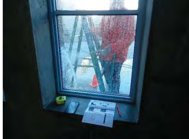
Photo No. 106 - Depicts the test specimen as viewed from the interior mid-test. BET&R's testing technician is visible outside applying the 25 psi controlled-spray at a distance of approximately 12 to 18-inches from the window target zone. BET&R utilized infrared thermographic imaging to confirm that no bulk water had penetrated the fenestration unit.
