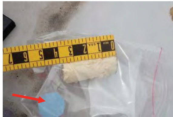
Photo No. 25 - Depicts the roof test cut sample extracted during this 2020 site visit, which revealed: One 4-inch-thick layer of mechanically-attached, organic/inorganic paper-faced polyisocyanurate roof insulation that is covered by a weathered, aged, chalky, and embrittled, single-ply Hypalon roof membrane, as was once manufactured in the U.S. by JP Stevens (See arrow indicating light-blue backside of roof membrane, the color utilized solely by JP Stevens on their Hypalon roof membranes).
