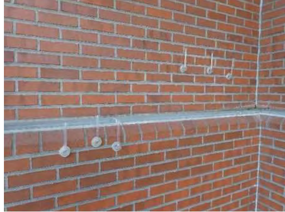
Photo No. 94 - Depicts an overview of testing conducted to the west of the Main Entrance at the North Elevation. Although the cluster of RILEM Tubes to the right was near an apparent location of moisture drainage from the sheet metal roof above, it performed approximately the same as the area to the left, just below the painted-steel support plate.
